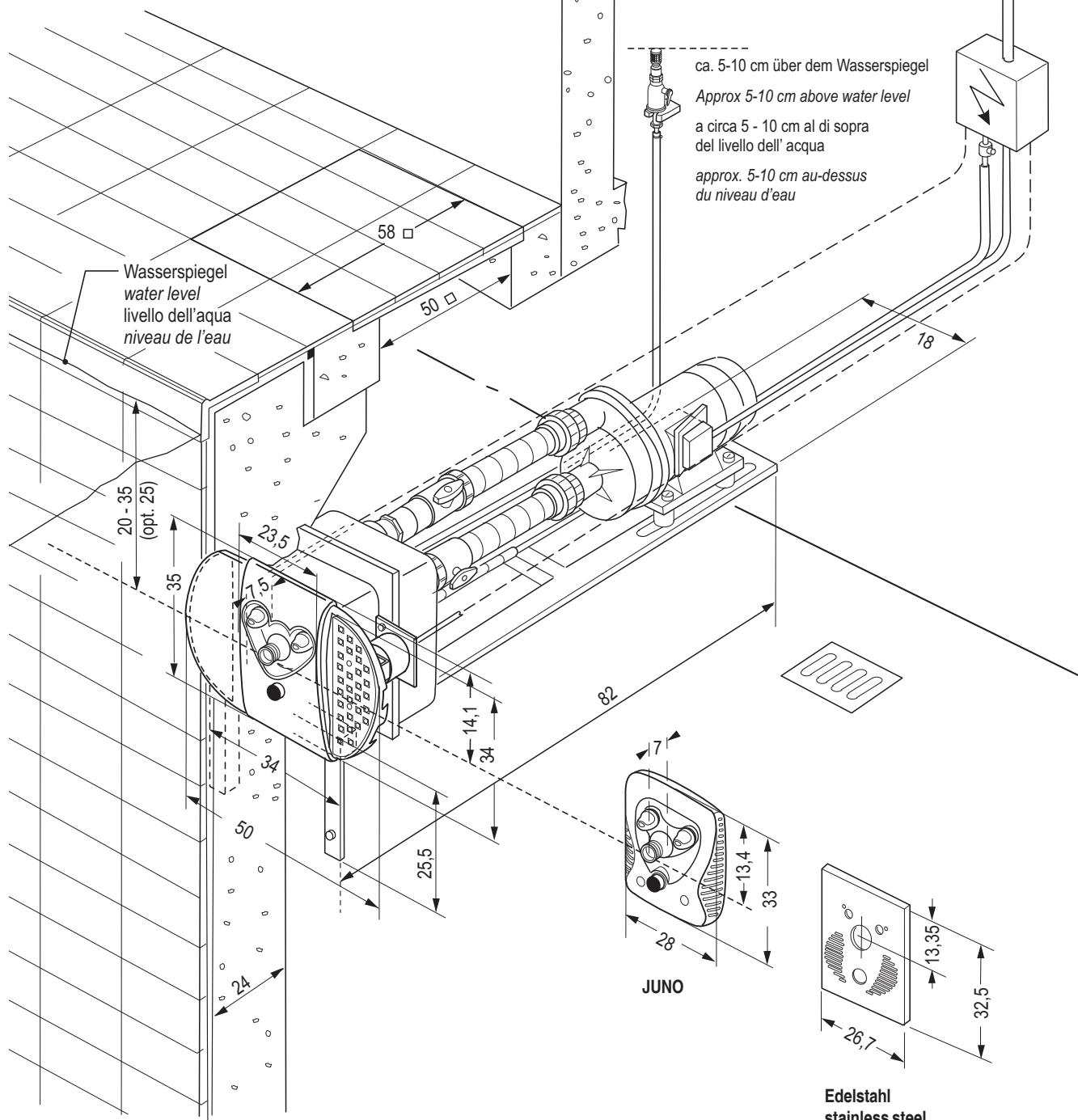
Abmessungen in cm / dimensions in cm / mesures en cm / quotazioni in cm
