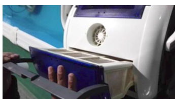
7. Slide the filter tray along the groove
