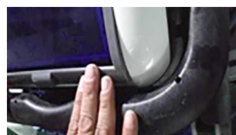
8. Press the two ends of handle to fix with robot
