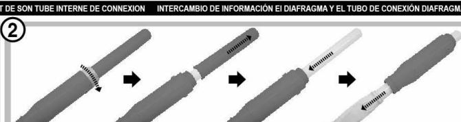
GB | Unscrew the screw cap of diaphragm chamber "C" and take it out. Take out the chamber extension tube and push the inside tube (diaphragm connection tube) forward to expose diaphragm completely. Hold the inside diaphragm connection tube (instead of diaphragm) to pull it out completely.
