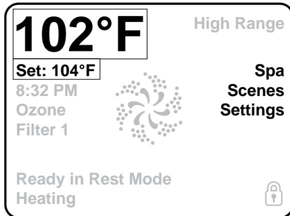
The only item that can be changed on the left side of the Main Screen is the Set Temperature. Touch either the set temperature line or the water temperature to go to the Set Temperature screen. See next page.
