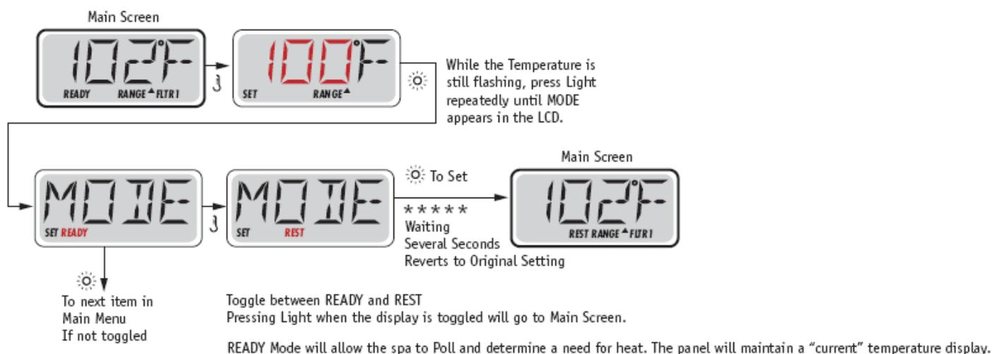
REST Mode will not Poll and will only heat during filter cycles. The panel will not display a current temperature at all times.
