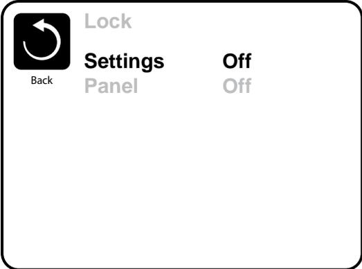
The control can be restricted to prevent unwanted use or temperature adjustments.
