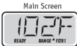
Waiting Several Seconds in the Main Menu will allow the display to revert to the Main Screen. Most changes are not saved unless Light ☀ is pressed. Refer to Key above.
