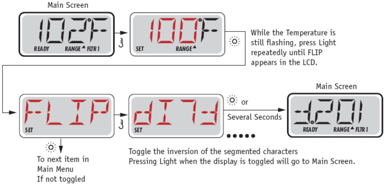
**Note:** Some panels may have a dedicated FLIP button, which allows the user to flip the display with a single button-press. The FLIP menu/functionality depends on Manufacturer configuration and may not be available. (Menu Style 1)
