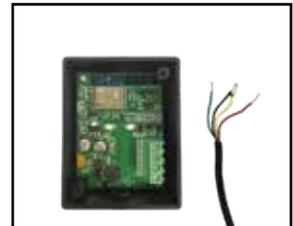
4. Discard the old cable tie and pull the cable out through hole. Keep the circuitry exposed, as the cable will need to be rewired back into place.
