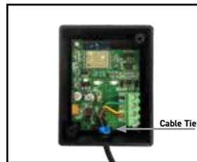
**3.** Gently pull any slack back through the hole and secure the cable tightly in place with the cable tie.
