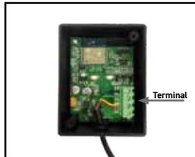
2. Release the 4 wires by loosening the terminal screws.
