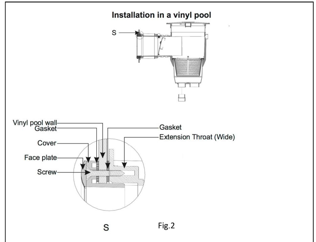
Ensure that the pool water level is constant and  $\frac{3}{4}$  parts of the skimmer is submerged in the water. This avoids air suction into the circuit that can damage the filtration pump.
