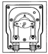
The principle of operation of the peristaltic pumps is based on pressure and subsequent release of the inner tube (A) by the roller (B) mounted on the roller-holder (C), which is driven by the motor.
