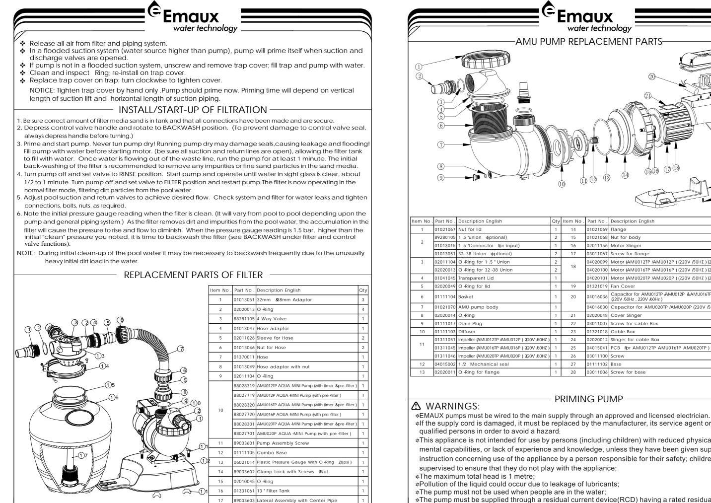
\*Pollution of the liquid could occur due to leakage of lubricants; \*The pump must not be used when people are in the water: \*The pump must be supplied through a residual current device(RCD) having a rated residual operating current not exceeding 30 mA.
