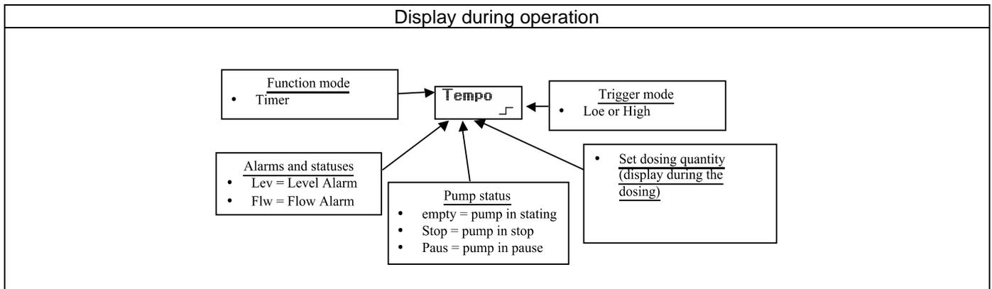
Paragraph 8 – Timed Dosage (**Frequency signal input “TRIGGER” not activated**)
