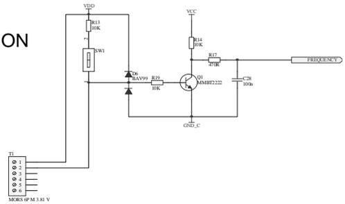
Connection diagram for frequency input with voltage signal
