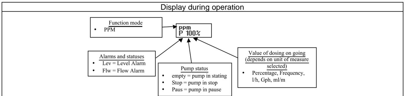
Paragraph 8 – Timed Dosage (**Frequency signal input “TRIGGER” activated**)
