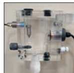
Probe for free chlorine
