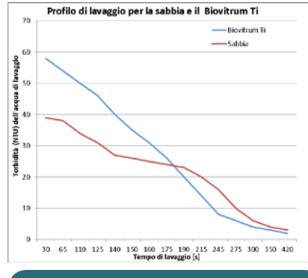
The curve shows the comparison between the backwashing water in a sand filter and a Biovitrum Ti one. The Biovitrum Ti filter expels up to 35% more impurities.
