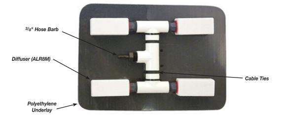
The diffusers included as part of the **ALP4** assembly are made of glass-bonded silica, are virtually indestructible and will give many years of service. The diffuser manifold comes with a polyethylene underlay to prevent the disturbance of sediments. The manifold is attached to the underlay with two polyethylene cable ties (included).
