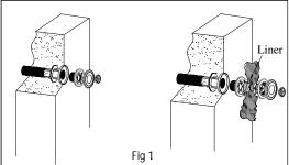
The suction nozzles can be assembled with threaded wall conduit 2" or assembly the connections 50 mm with PVC glue.
