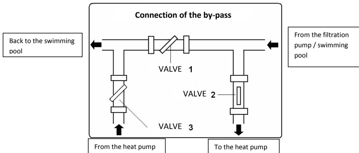
The heat pump is equipped with 2 threads enabling the connection of input and output fitting (d50). For connection with the filtration circuit use the d50 PVC pipe or 50/38mm adapters (6/4"). Please refer to *section 3.4 Description of the basic parts* in order to make sure which thread is water input and which water output. It is advised to apply lubricating oil on threads before tightening the connection.
