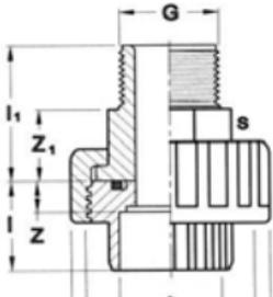
Picture: Hose nut with external thread PN16.
