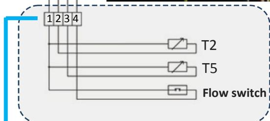
Picture: Power supply connection of the condensing unit, auxiliary circulation pump and 1-4 sensors of the water unit (above).
