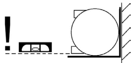
Picture: Installation of water unit without box – levelled with spirit level.
