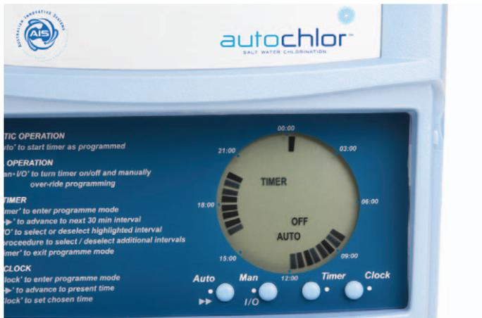
All segments between the start and stop times need to be turned ON (darkened) as shown in the above picture.
