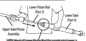
NOTE: Head of Lower Piston Rod fits snugly into Lower Tube. Some pressure may be needed to insert.
