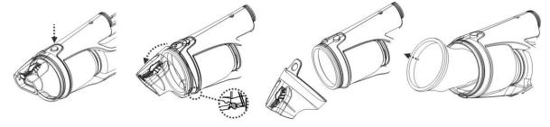
**CAUTION!** Replace the damaged filter bag immediately before the next operation.
