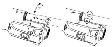
To release the telescopic pole, press down the side pins simultaneously and pull out the pole.
