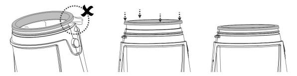
To re-install the canister, first align the notch of the canister with the hook on main body and then press the canister onto main body. Make sure the locking hole on the clear canister is secured with the locking button.
