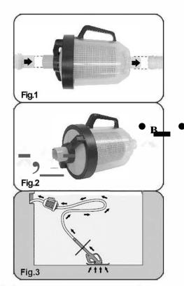
ATTENTION: Canister may trap air if it is exposed. This may cause a loss of suction power, which can cause cleaner to move slowly or even fail to climb walls.
