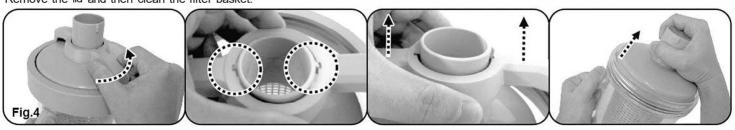
Reverse the steps to reinstall the unit. Make sure the lid O ring is in place.
