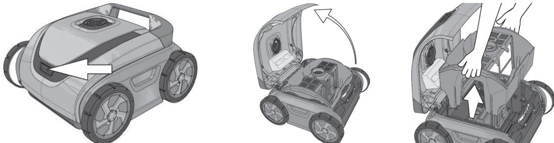
3. Flip the bucket assembly over to remove the debris and then rinse with a garden hose to remove small particles.
