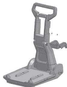
Insert Lower Hook using 2 self-tapping screws
