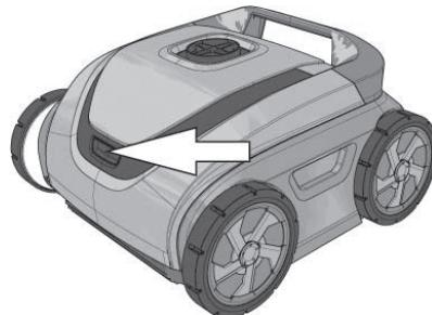
7. Close the dome and press the lid button to snap dome into place.
