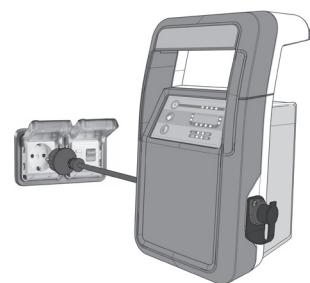
7. The power indicators should be slowly pulsing. This means that the power supply is in standby mode.
