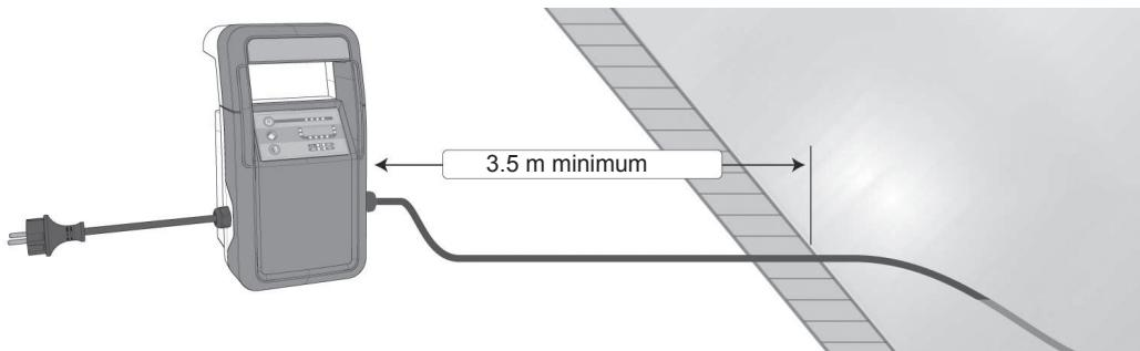
3. Stretch out the floating cable along the pool deck in the sun to remove any twisting the cord has from storage and measure out the approximate amount of cleaner cord needed for pool coverage.
