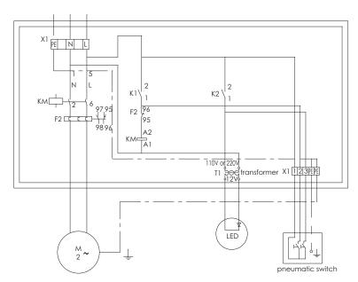
220V/50Hz, 110V/60Hz counter current jet circuit diagram
