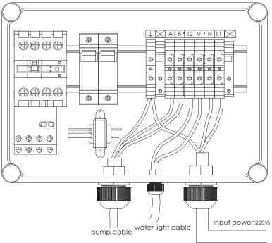
220V/110V control box wiring diagram
