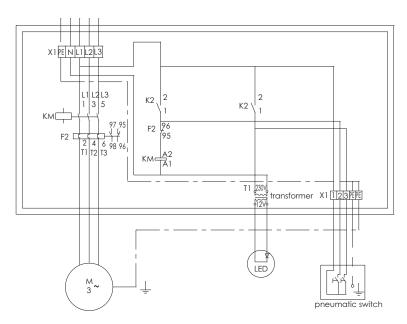
380V/50Hz counter current jet circuit diagram
