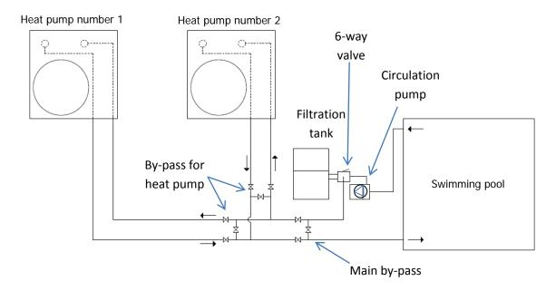
By multiple heat pump connection it is possible have all the heat pumps **always on** and running when heating / cooling is required **or** to have the heat pumps **gradually turning on and off** so at certain conditions (e.g. when requested water temperature is few degrees off the current water temperature) not all the heat pumps would run. Gradual turning on and off is achieved by setting the different requested water temperatures on multiple heat pumps. For example:
