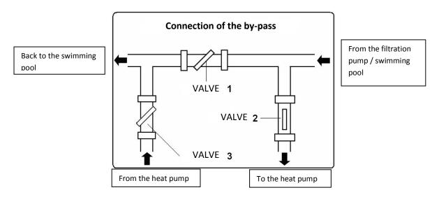
The heat pump is equipped with 2 threads enabling the connection of input and output fitting (d50). For connection with the filtration circuit use the d50 PVC pipe or 50/38mm adapters (6/4"). Please refer to section 3.4 Description of the basic parts in order to make sure which thread is water input and which water output. It is advised to apply lubricating oil on threads before tightening the connection.
