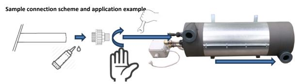
Picture: Sample water connection to the heat pump. Flexible hose glued onto hose nut adapter with external thred that is tightened into the heat pump exchanger thread. Picture is illustratory.
