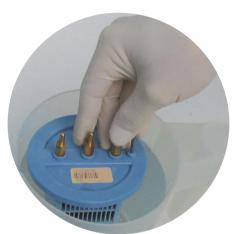
There will be a reaction as the calcium is dissolved. When the reaction ceases (about 10 minutes) rinse the electrode in clean water, wipe the brass terminals dry and check that all calcium has been dissolved. If not, repeat the process with a new solution.
