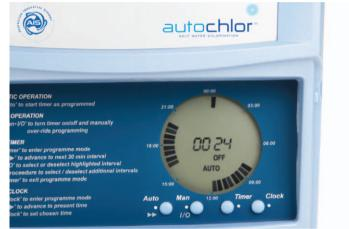
Press the "Auto" button to put the chlorine generator into automatic timed operation. The word AUTO, the time of day and your programmed times will appear on the screen. The chlorine generator and the filter pump will turn on and off at the times you entered during programming.
