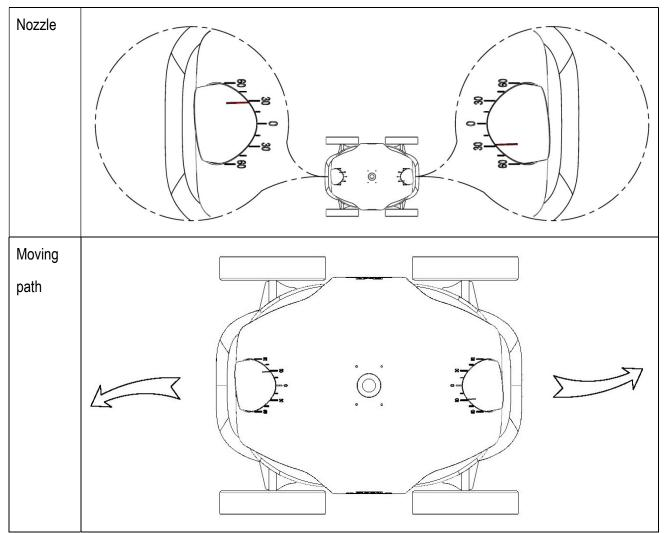
Setting 7:  $45^{\circ}$  /  $45^{\circ}$  When the cleaner does not have full coverage of pool by setting 6, and need to move in more curved line.
