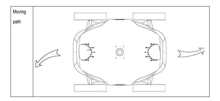
Setting 5: 30  $^\circ~$  / 60  $^\circ~$  Cleaner moves in more curved line than setting 4.
