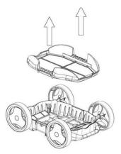
Wash the filter tray and chassis then reassemble the cleaner
