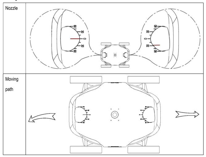
Setting 4: 15  $^\circ\,$  / 60  $^\circ\,$  when the cleaner need to move in more curved line to cover the pool
