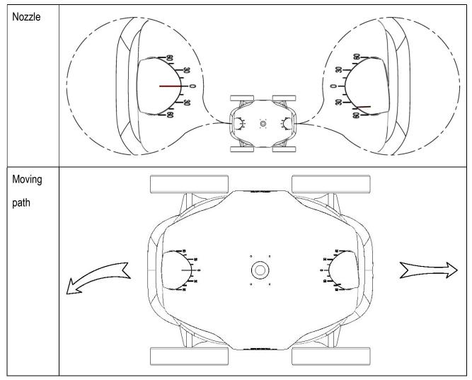
Setting 3;  $0^{\circ}/30^{\circ}$ , When the cleaner still moves in too much curved line to cover the pool by above settings.
