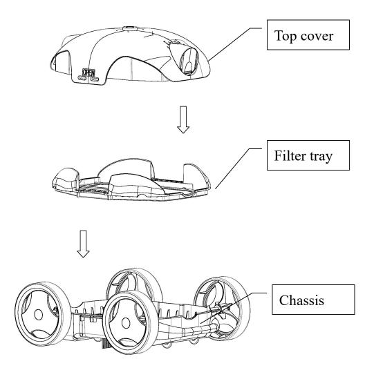
Assemble the cleaner according to above structure
